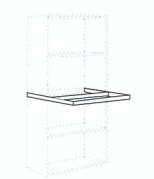
Telaio scorrevole portacartelle per librerie modulari Extractable frame on telescopic runner for modular storage units
